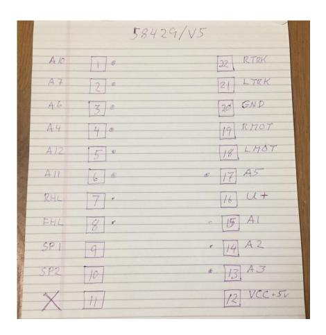
This is the labeled 21-pin connector pinout diagram for a 12-output decoder. Combining some functions for an 8-output decoder works well also.
