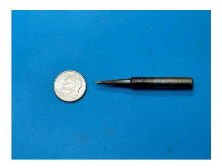
The Weller wlc100 40-watt soldering station with the original chisel tip and a Weller ST-7 soldering tip are enough to build an entire railroad and solder all your decoders if you are careful with the tips. Only the Weller tips hold up well. All can be found on eBay and elsewhere. It doesn't have to be this soldering iron. A 40 watt adjustable soldering iron with a fine tip for electronics and a chisel tip for track is what I recommend.
