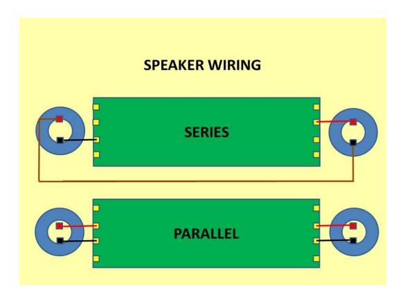
This is one way to set up series of parallel speakers in your locomotive with a large Decoder Buddy.
